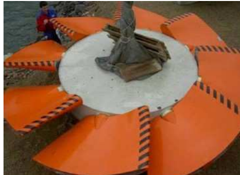
Figure 21 – VLH DN 4500 runner of the Millau demonstration site
